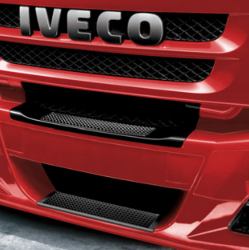
Illuminated non-slip steps for getting into the cab easily and safely.
