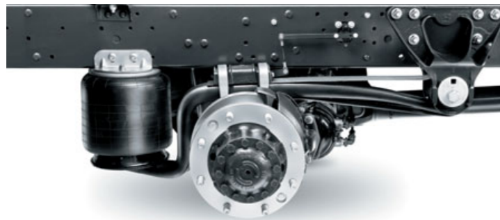
Air rear suspension with 2 air springs for versions from 6 to 14 t
